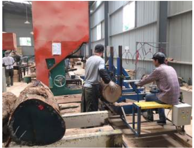
Chinese sawmills use bandmill equipment that was smaller in scale than U.S. mills. The logs were cut into 1, 2 and 3-meter lengths before sawing. The cants and lumber were moved by hand from each station and packing for kilns. Below are sorted packs.
