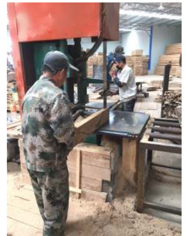
Chinese sawmills use bandmill equipment that was smaller in scale than U.S. mills. The logs were cut into 1, 2 and 3-meter lengths before sawing. The cants and lumber were moved by hand from each station and packing for kilns. Below are sorted packs.
