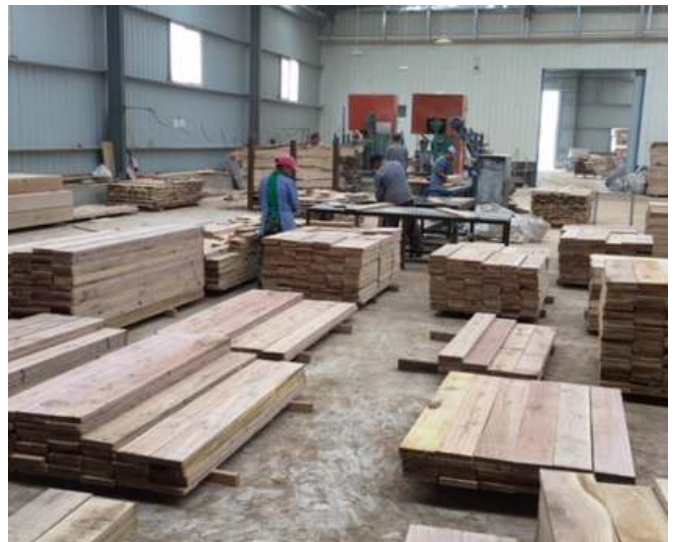
Chinese sawmills use bandmill equipment that was smaller in scale than U.S. mills. The logs were cut into 1, 2 and 3-meter lengths before sawing. The cants and lumber were moved by hand from each station and packing for kilns. Below are sorted packs.
